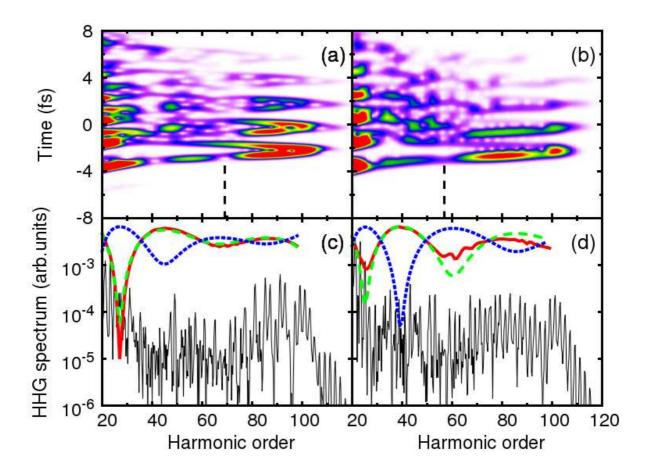
Figure 4: (Color online) Time-frequency analysis and HHG spectra of  $H_2$  for the laser intensity  $2\times 10^{14}\,\mathrm{W/cm^2}$ . Also shown are the emission spectra obtained using the recollision model, Eq. (9), with the ionization phase from Figure 3 (thick solid lines),  $\phi=\pi$  (thick dashed lines) and  $\phi=0$  (thick dotted lines). Left panel:  $R=5.2\,\mathrm{a.u.}$  Right Panel:  $R=6\,\mathrm{a.u.}$
