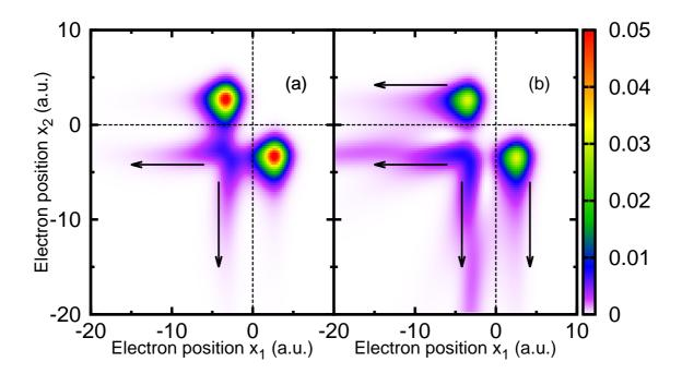
Figure 2: (Color online) Two-electron density at the peak of a half-cycle pulse for R=6 a.u. (a) Laser intensity  $2\times10^{14}$  W/cm<sup>2</sup>. (b) Laser intensity  $4\times10^{14}$  W/cm<sup>2</sup>.
