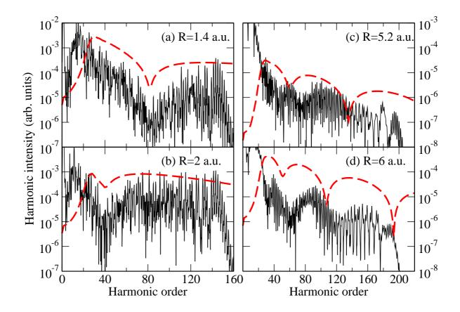
Figure 1: (Color online) HHG spectra for 1D  $H_2$  at various internuclear distances. The laser intensity is  $3 \times 10^{14} \, \text{W/cm}^2$  in (a),(b) and  $4 \times 10^{14} \, \text{W/cm}^2$  in (c),(d). Dashed lines: spectra emitted by collision of a Gaussian wave packet with the molecular ion.
