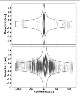
**Figure 1.** Husimi electron distribution around an argon (Ar) atom (top) and an Ar + Ar<sup>+</sup> ion system (bottom). Laser intensity  $I = 1 \times 10^{14}$  W cm<sup>-2</sup>. The solid line represents the zero-energy boundary, outside of which the parts of electron distribution can be considered ionized.
