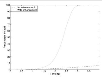
**Figure 3.** The percentage of argon cluster surface area ionized, plotted as a function of time. The dashed line corresponds to the case for no enhancement ( $K_{i,k}=1$ ), whereas the solid line includes enhancement. Laser parameters are  $I=5\times 10^{13}$  W cm<sup>-2</sup> and  $\lambda=800$  nm.
