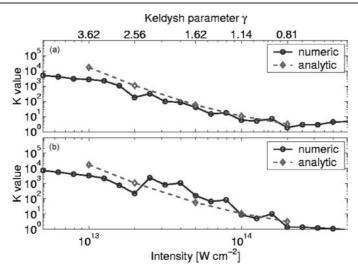
**Figure 2.** K values given by numerical simulations in relation to the SFA theory for a trapezoidal 1-20-1 pulse ( $\lambda = 800$  nm) for argon cluster. Top plot gives comparison where, numerically, the effective field produced by the ion is a homogeneous DC field. Bottom plot has the ion field modelled by the soft-core potential.
